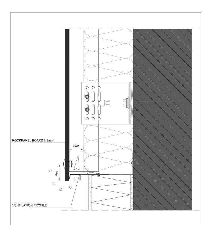
\* FOR ALUMINIUM CONSTRUCTIONS IN AN OPEN FACADE ROCKPANEL GROUP RECOMMENDS A CAVITY DEPTH OF 40 - 100mm
