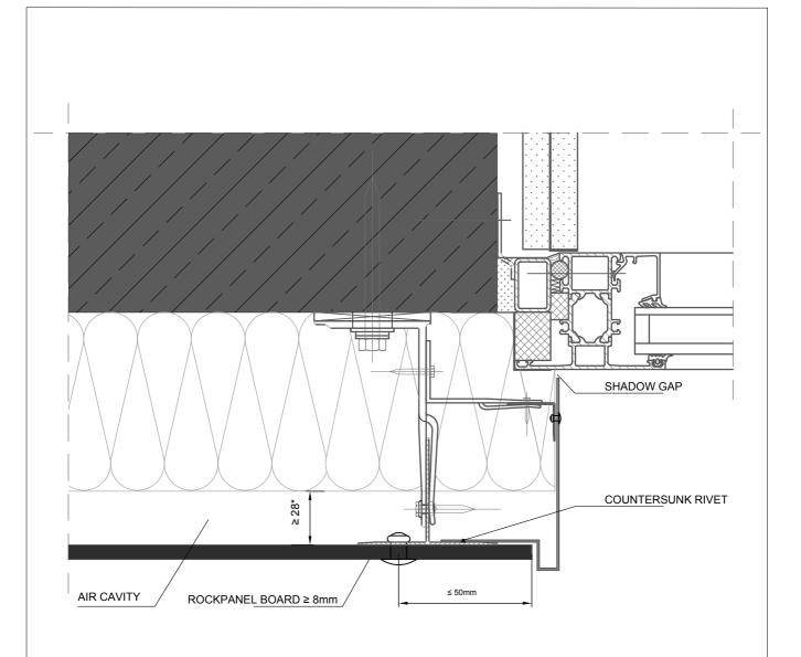
\* FOR ALUMINIUM CONSTRUCTIONS IN AN OPEN FACADE ROCKPANEL GROUP RECOMMENDS A CAVITY DEPTH OF 40-100 mm
