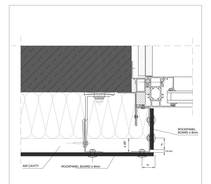
\* FOR ALUMINIUM CONSTRUCTIONS IN AN OPEN FACADE ROCKPANEL GROUP RECOMMENDS A CAVITY DEPTH OF 40-100 mm
