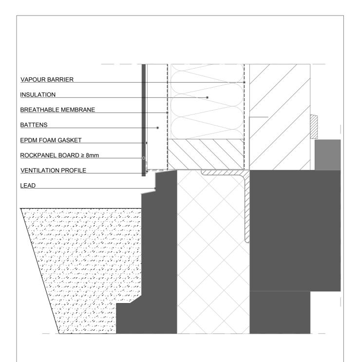
\* START ROCKPANEL BOARD ABOVE HARD SOIL ≥ 20mm / SOFT SOIL ≥ 50mm
